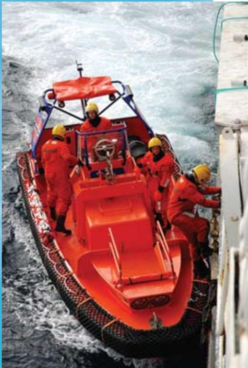
**Fig 1 - Norwegian Coastguard boarding vessel with twin HamiltonJet HJ274 waterjets**
