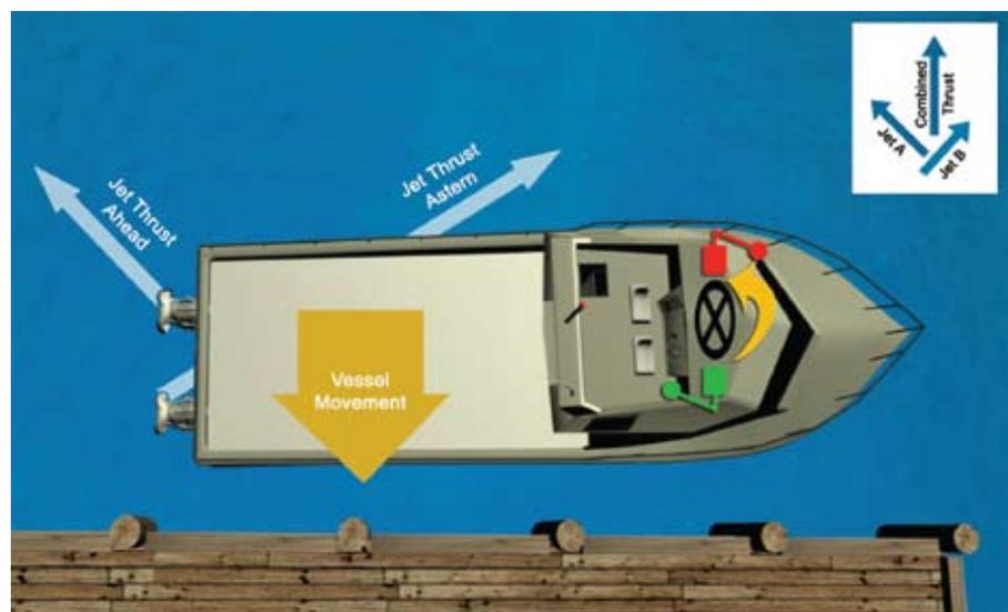
Fig 4. The resulting sideways movement when twin waterjet thrust is vectored appropriately.
