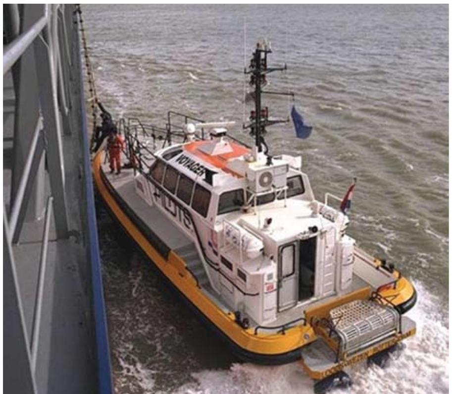
**Fig 6. Dutch Pilot Vessel picking up a pilot and positioning its stern to quickly pull away from a ship.**
