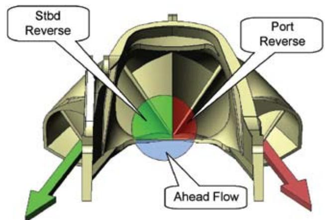
**Fig 2. HamiltonJet split duct reverse deflector as viewed from jet steering nozzle.**
