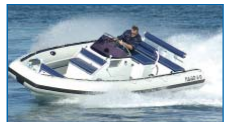
A 6m pleasure boat/tender with single Hamilton HJ213 waterjet from Naiad, New Zealand
