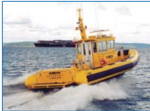
This SeaTow rescue/recovery RIB is also used as a pilot boat in Brunswick, GA, USA. It's an Almar RAV powered by twin HJ274 waterjets.
