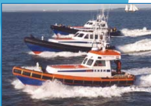
Waterjet-powered rescue RIBs of the KNRM (The Netherlands)
