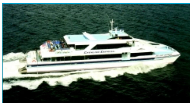
Quad Hamilton Model HM651 Waterjets pushed Jet Cat Express to over 40 knots during sea trials.
