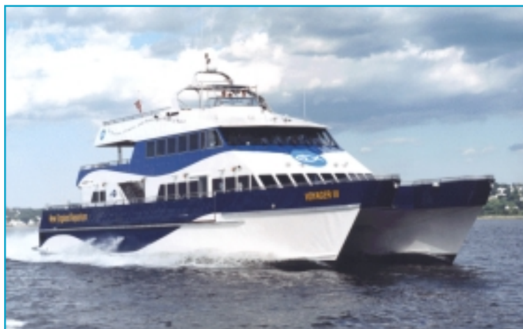
34 metre Catamaran Ferry "Voyager III", Boston Harbour, USA Quad Hamilton Model HM461 Jets
