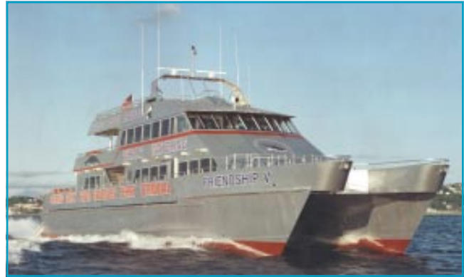
Bar Harbor Whale Watch Co's 34 metre INCAT Catamaran Ferry "Friendship V" – Quad HM461 jets, 35 knots
