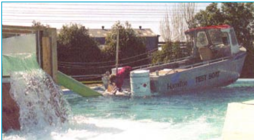
Seven-metre Hamilton Jet Test Boat undergoing flow calibration tests.
