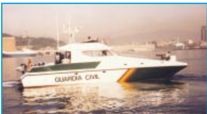
Spanish Civil Guard Patrol Craft 40 knots with twin HJ362 waterjets
