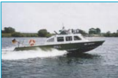
Example of a well trimmed planing monohull – 13.4m customs Patrol craft with twin 362 jets
