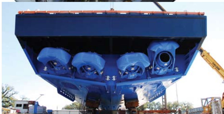
Top: Installing the HT900 waterjets in Aaron S McCall Bottom: The quad HT900 lineup
