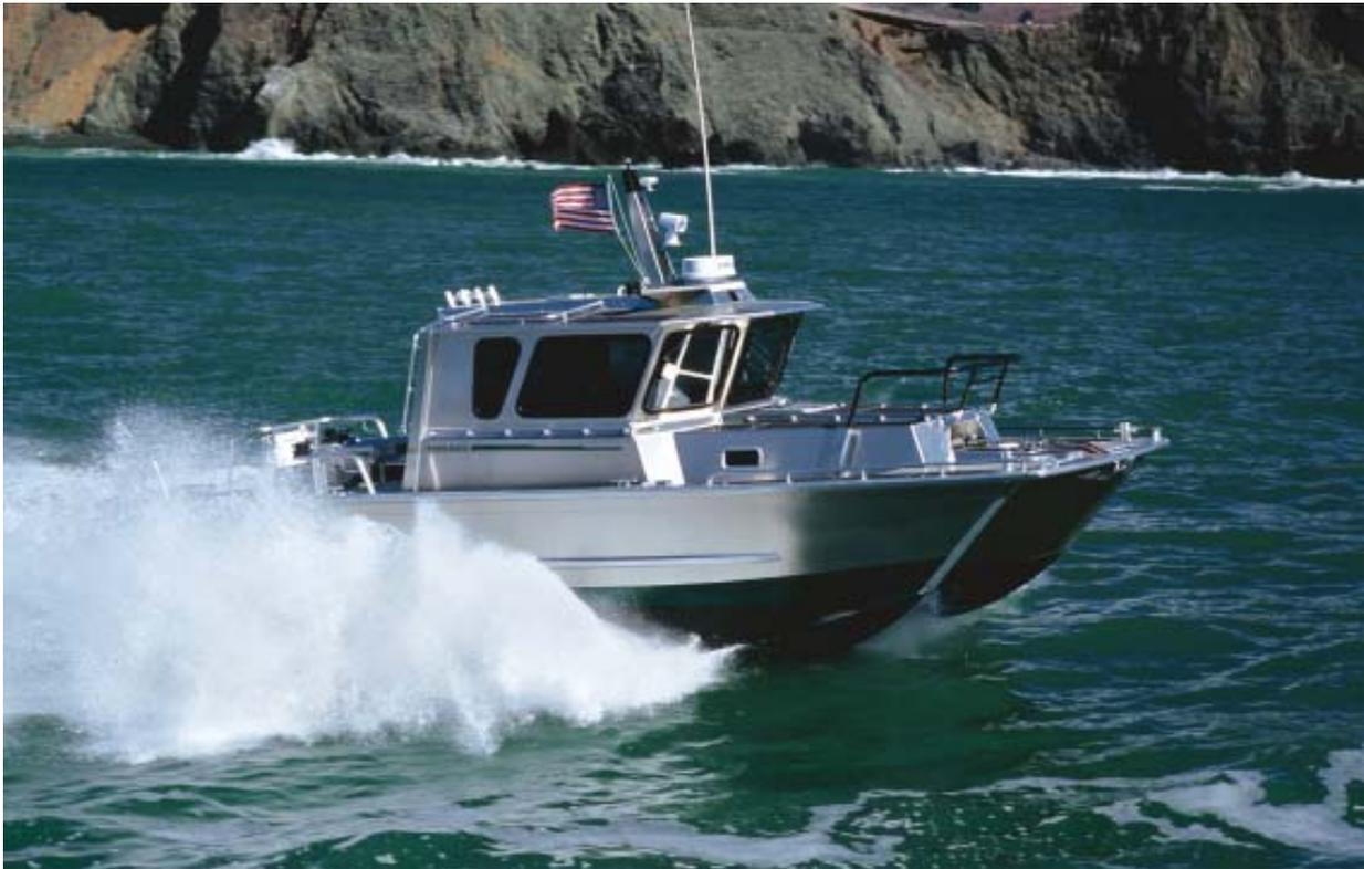
**New California-based boat builder, Moose Boats, unveiled its first innovative vessel at the New Orleans Work Boat Show in late 2001. The 'Moose J3200' combines Hamilton Waterjet propulsion in a 10-metre symmetrical catamaran hull, and is specifically designed to be operator friendly and rugged, and offer value for money in a variety of roles.**
