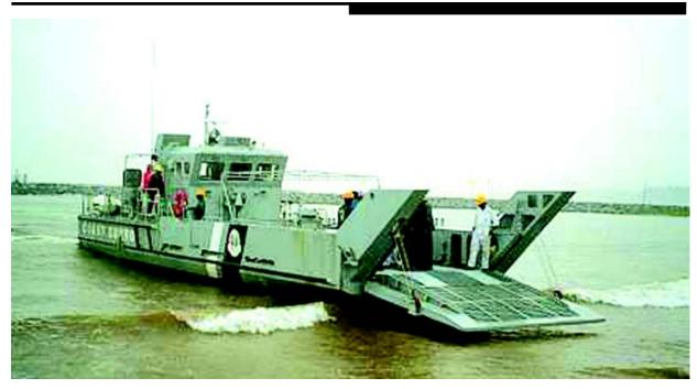
The National Security Service of the Republic of Maldives have taken delivery of a new Hamilton Jet powered landing craft. Twin Model HM422 jets directly driven by MAN diesel engines push the aluminium craft to speeds over 20 knots when fully laden.
