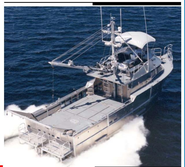
"The Surveyor" is to be used for underwater exploration and recovery work. Quadruple Hamilton 32 I produce thrust for a top speed of 44.5 knots so work sites can be accessed quickly. With one propulsion system shut down, speeds over 30 knots can be maintained. A Hamilton HSRC jet control system gives precise manoeuvrability at all speeds and shallow
