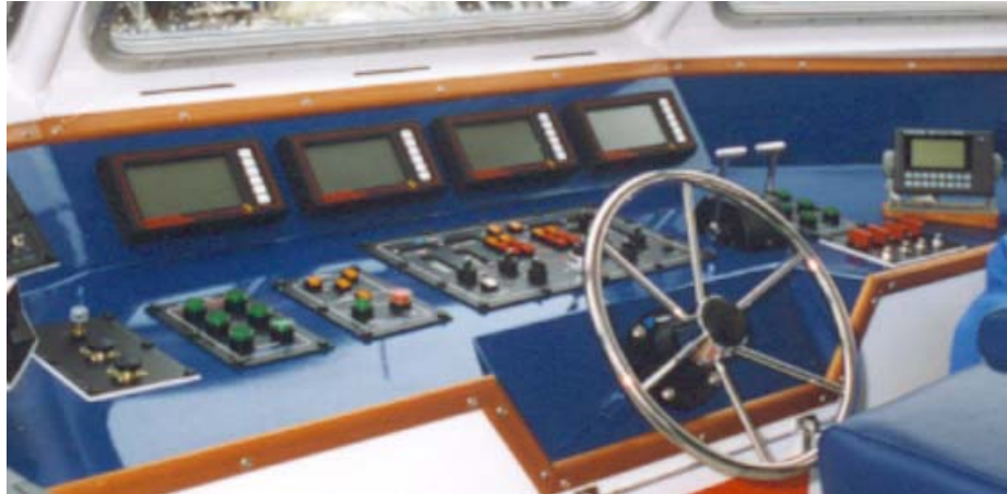
Main Forward Racing Helm Station (Primary Controls are Repeated Facing Aft)
